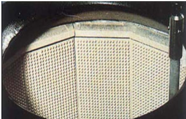
Exhibit 8: Radiant panel installed in gas crucible furnace
