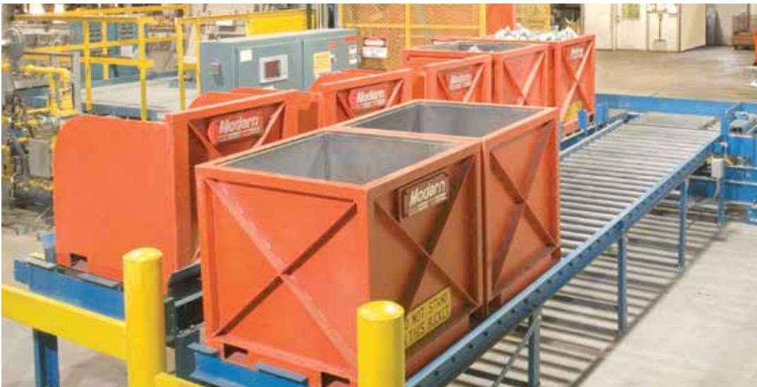
Scrap and ingot buckets on automated material handling conveyor
