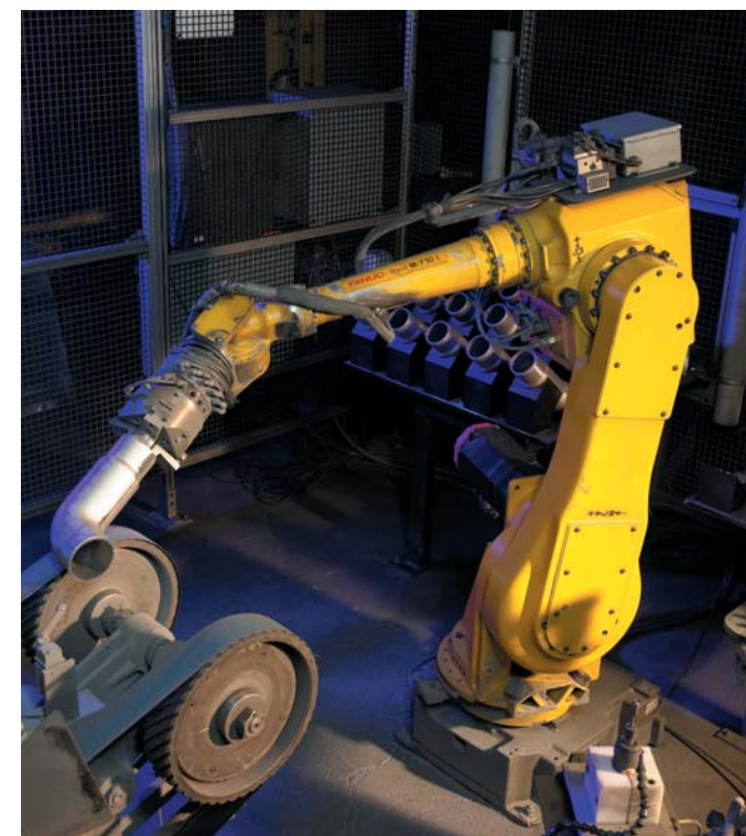
Above: Wisconsin Aluminum utilizes state-of-the-art coordinate measuring machine (CMM) technology to verify dimensional accuracy of its customer's castings. Below: Wisconsin Aluminum employs robotic sanding technology at its facility. This investment has generated improvements in productivity and quality.
