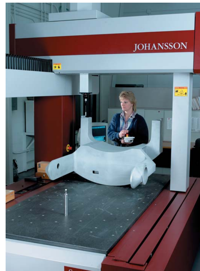
Above: Wisconsin Aluminum utilizes state-of-the-art coordinate measuring machine (CMM) technology to verify dimensional accuracy of its customer's castings. Below: Wisconsin Aluminum employs robotic sanding technology at its facility. This investment has generated improvements in productivity and quality.
