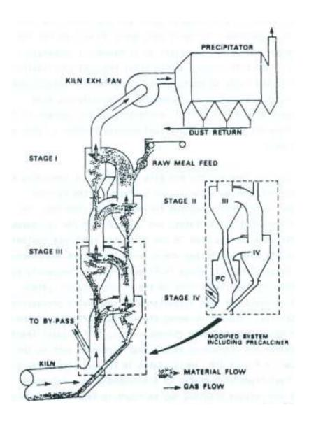
Figure 3-11. Suspension Preheater Used in the Cement Industry
