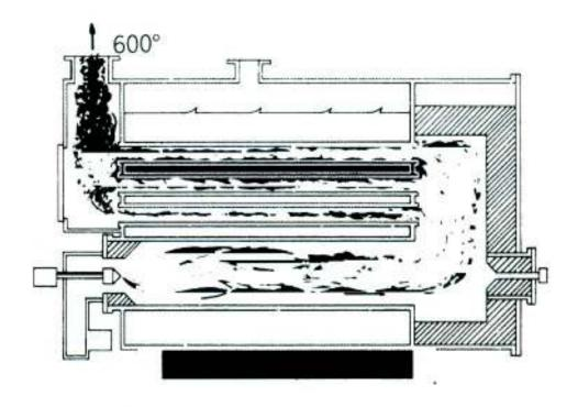
Figure 3-4. A Two-Pass Firetube Boiler (Reference 3-7)
