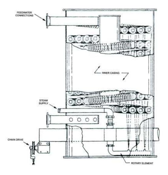
Figure 3-3. A Cylindrical Economizer with Rotary Sootblower (Reference 3-4)
