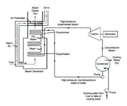
Figure 3-2. A Schematic Diagram of a Steam Power Plant (Reference 3-3)
