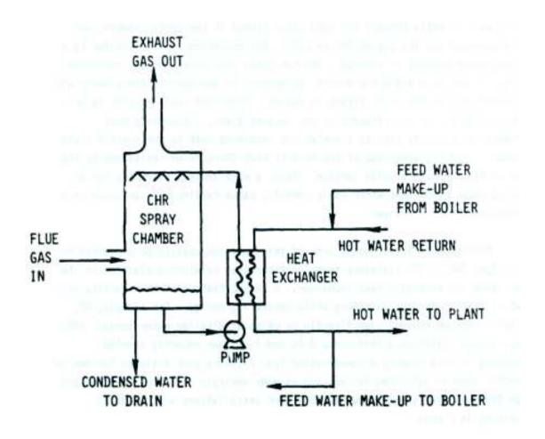
Figure 3-12. Low-Temperature Direct Contact Heat Exchanger (Reference 3-25)
