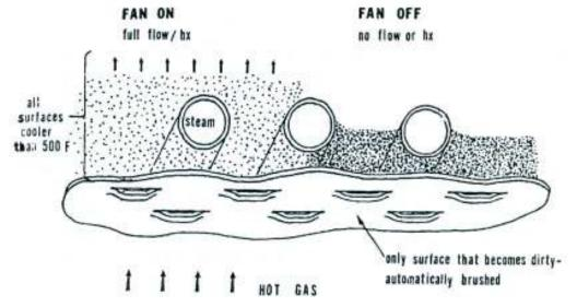
Figure 3-13. A Schematic Drawing of a Fluidized Bed Heat Recovery System (Reference 3-29)
