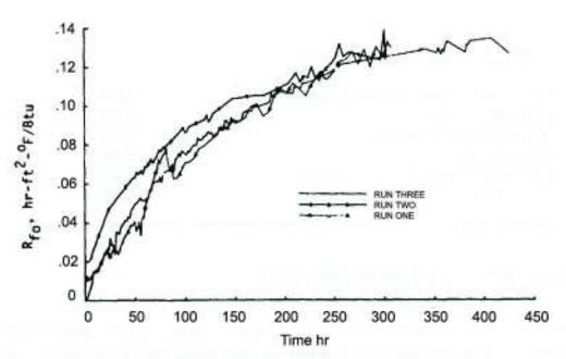
Figure 4-1. Experimental Diesel Exhaust Fouling Resistances, Henslee and Bogue (Reference 4-5)
