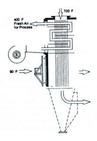
Figure 3-6. A Gas-to-Air Heat Exchanger Used in the Cement Industry (Reference 3-8)
