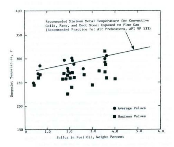
Figure 3-15. Acid Dewpoint Temperature of Combustion Gases
