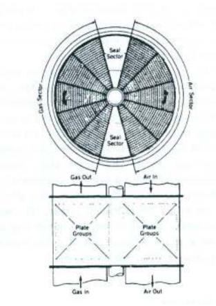
Figure 3-10. The Rotary Generator (Reference 3-22)
