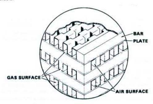
Figure 3-9. Plate-Fin Heat Exchanger Construction (Reference 3-18)
