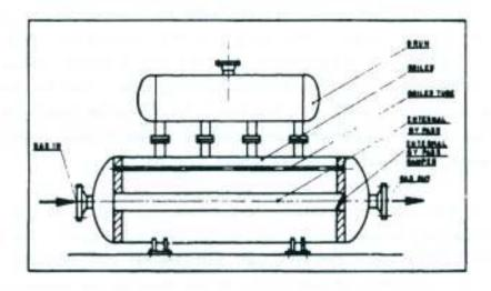
Figure 3-5. External and Internal Bypass in Firetube Boiler for Exit Gas Temperature Control (Reference 3-1)
