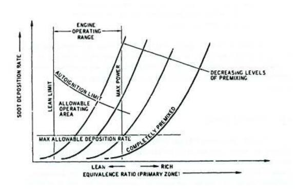
Figure 6-1. Probable Soot Deposition Rates with Combustion System Parameters (Reference 6-2)
