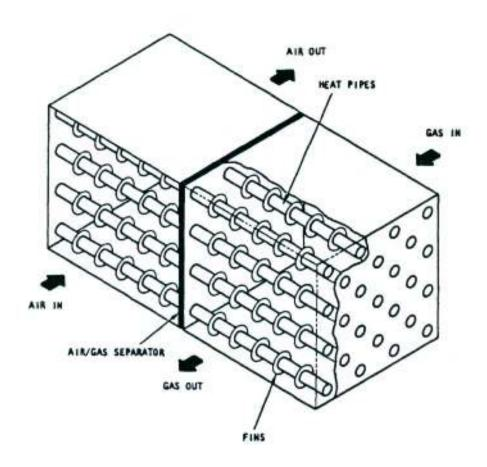
Figure 3-14. Schematic Drawing of a Heat Pipe Heat Recovery System (Reference 3-31)
