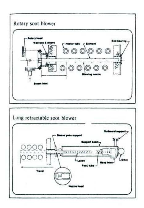
Figure 6-2. The Rotary and Long Retractable Sootblowers (Reference 6-7)
