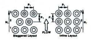
Figure 3-8. A Comparison of Inline Versus Staggered Layouts (Reference 3-10)
