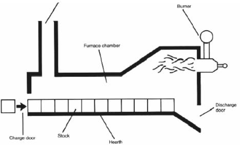
Figure 1: Typical Furnace Components (The Carbon Trust, 1993)
