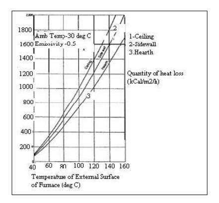
Figure 15. Relationship between Surface Temperature and Quantity of Heat Loss (BEE, 2005)
