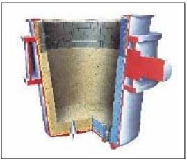
Figure 9. A Monolithic Lining for Ladel
